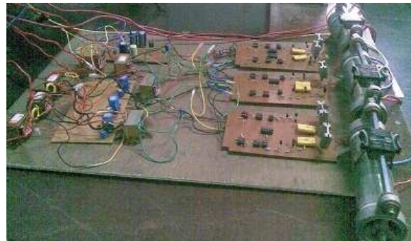
Figure 21. Fabricated three-phase ac voltage regulator using IGBT.
