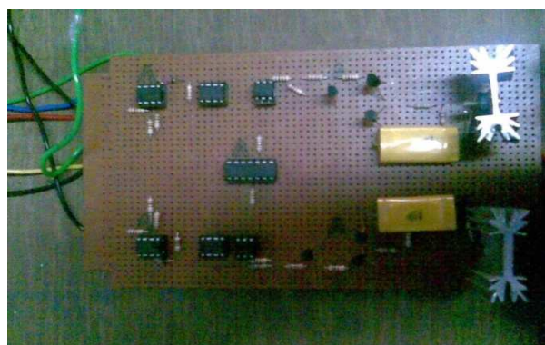
Figure 19. Fabricated single-phase soft starter
